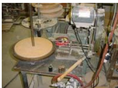
Indexing drilling station
